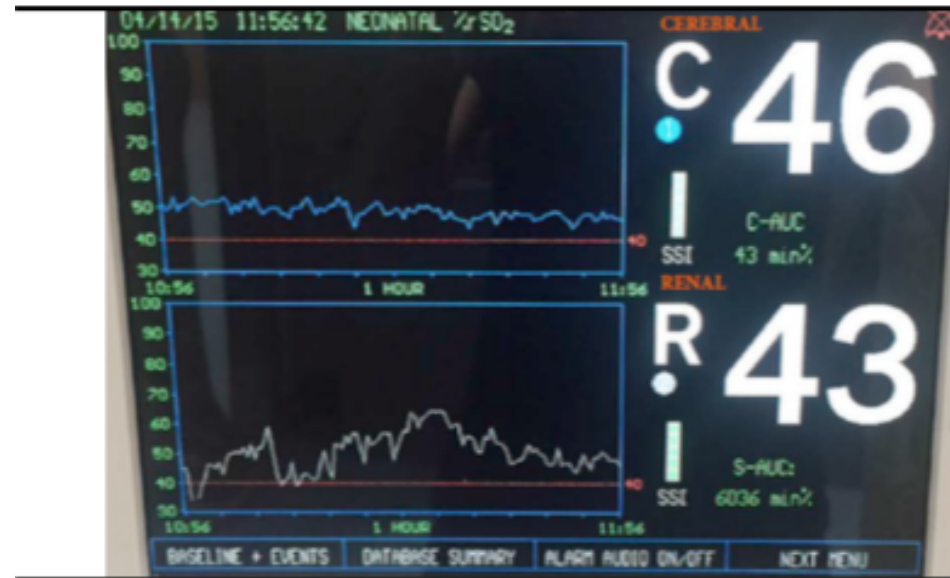
FIGURE 1. NIRS device monitor showing cerebral (C) and renal (R) SvO 2 trends over 1 hour.
